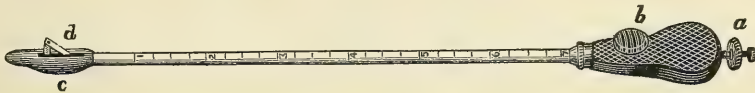
FIG. 622.—Dr. E. A. Banks's urethrotome. a , Screw-gauge. b , Sliding-knob. c , Bulb. d , Knife.
